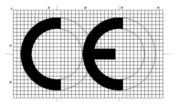
If the CE conformity marking is reduced or enlarged the proportions given in the above graduated drawing must be respected.
